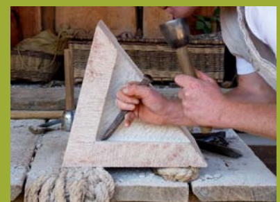
The final chiselmak on the final triangle-shaped coping stone.
