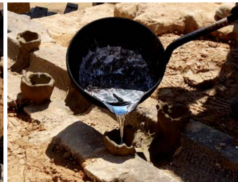
The molten lead is poured into a clay mould
