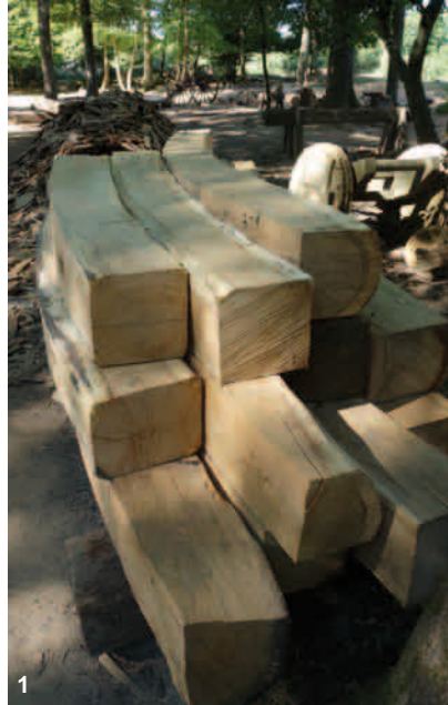
1: curved wall plates 2: straight wall plate of the cut-off inner wall 3: roof timbers stocked in the workshop
